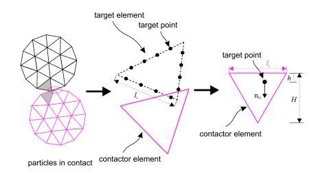
Figure 2. Schematic of contact interaction and contact force calculation.
