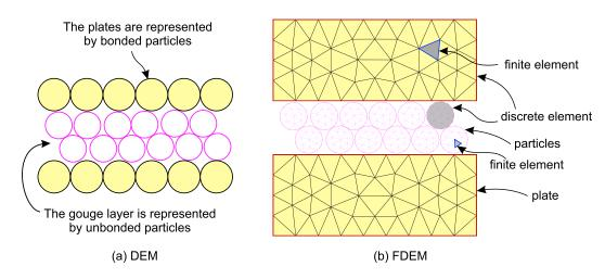
**Figure 1.** Numerical representation of the fault containing granular fault gouge using the discrete element method (DEM) and combined finite-discrete element method (FDEM). (a) In the DEM the plates are simplified by a set of bonded particles and the gouge layer is composed of a series of rigid particles. (b) In the FDEM the plate is explicitly represented and both plates and particles are further discretized into finite elements to capture their deformation and stress evolution.
