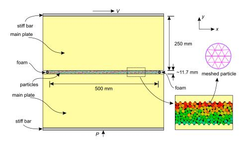
**Figure 3.** Combined finite-discrete element method (FDEM) model of the granular fault system and its geometrical dimensions. The top right inset shows the discretized particle used in the simulation that composed of 24 approximately equal size elements and its comparison with a circle.
